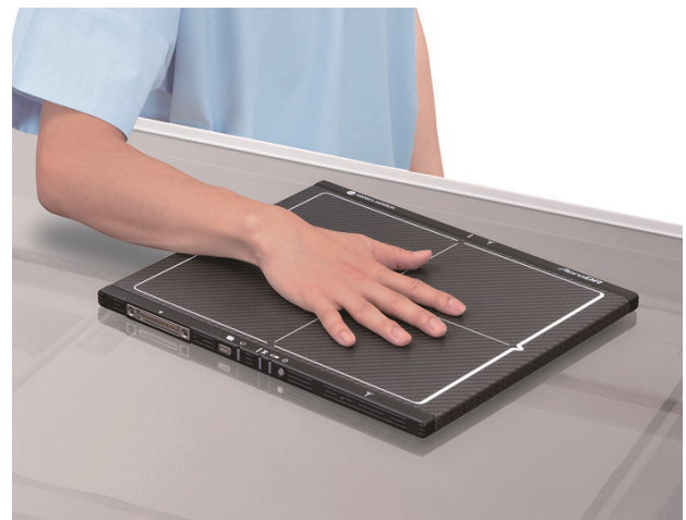
Fig. 5 World lightest (1.7 kg) 10×12 cassette: the AeroDR1012.
