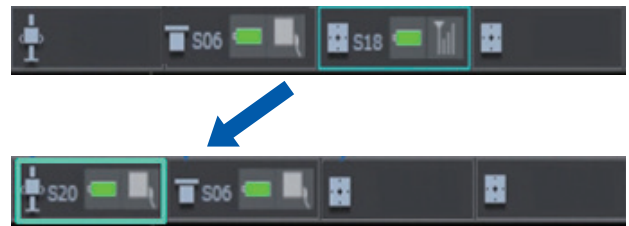
Fig. 4 The location of an AeroDR1717 cassette is automatically tracked by the CS-7 portable control station.
